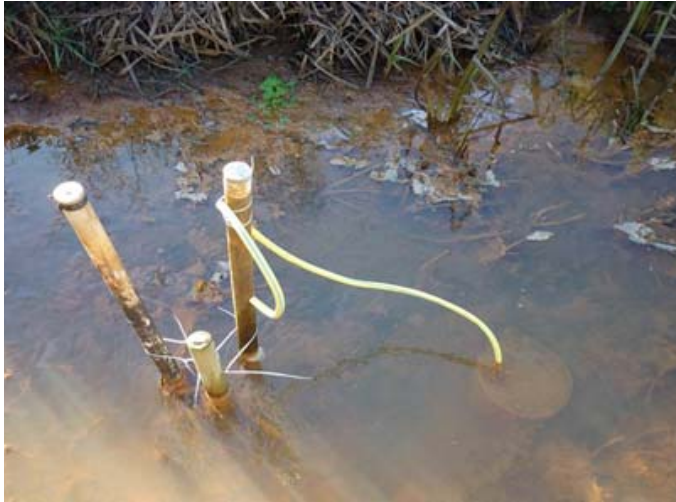
Figure 4. A piezometer nest comprising three piezometers, installed in different depths in the streambed to determine the hydraulic gradient and monitor pressure heads as well as water quality parameters. A seepage meter is installed to the right of the three piezometers.
