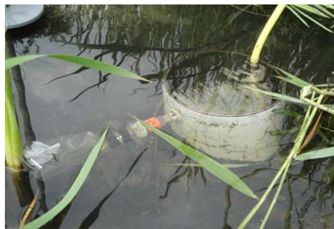
Figure 3. Half-barrel seepage meter installed in the bed of a lowland stream with a low flow velocity.
